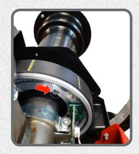
If these screws are black (ferromagnetic burnished steel), they must be replaced with other screws of the same size in non-magnetic STAINLESS steel (VTE M4X10).
